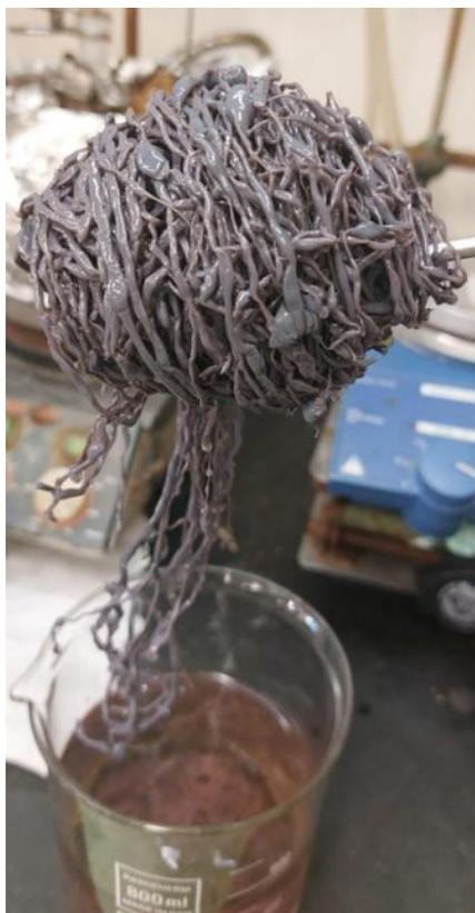
**Picture 2. Precipitate of the unoxidized precursor of sPPS-390-XXL in *i*-PrOH**
