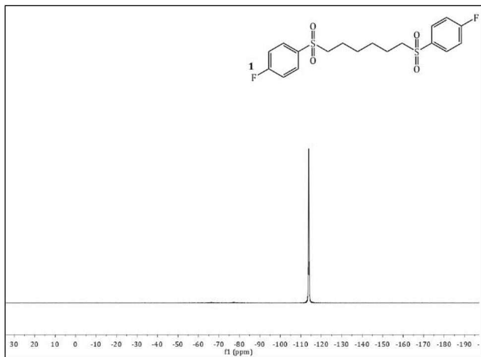
Figure 48.  $^{19}\text{F}$  NMR spectrum of FDPS-Hex-FDPS in  $\text{CDCl}_3$
